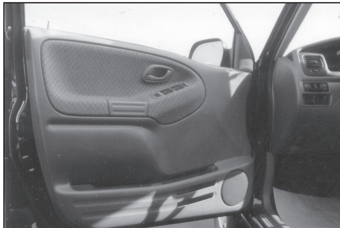
FRONT DOOR 7" 4-HOLE SPEAKER PROVISION.
