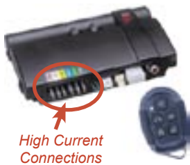
This is an example of an all inclusive remote starter where all the high current connections (at left of the controller) and the low current connections are contained in one chassis. The drawback is that it's larger and may be harder to find a suitable location.
