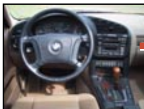
A DIN sized headunit in a 95 BMW 3 series means direct replacement
