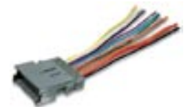
An Installation Harness for a GM vehicle. Note the color coded wiring. This is what the aftermarket headunit utilizes for a connection into the vehicle wiring.
