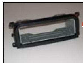
For non-DIN cars installing an aftermarket headunit, use an installation kit to mount the sleeve
