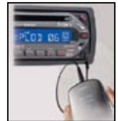
Many headunits have front panel AUX inputs to connect carry in audio devices easily. Rear panel RCA AUX inputs are also found on some models.
