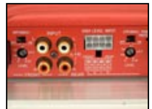
Many amplifiers feature both RCA and Speaker Level type inputs for increased flexibility.
