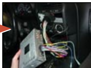
Aftermarket units install with only the mounting sleeve and installation wiring harness
