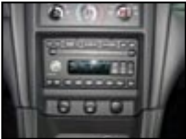
A Double DIN application in a 2003 Ford Mustang
