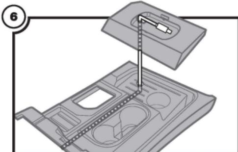
7. Use the provided two-sided adhesives to secure the panel/module from moving then connect the Qi module to the type-c connector. Once the module is connected place it into the bezel then reconnect everything in reverse order of the disassembly to complete the installation.
