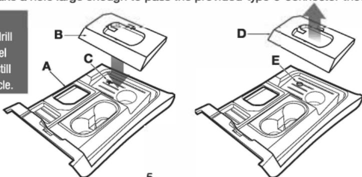
5. Connect the provided power t-harness according to the diagram displayed in the Test Connection box at the top of page 5 or illustrated at the right. Connect the female and male 12V power connectors first then route the type-c connector to the designated slot created during the preparation step at the bottom of page 5.
