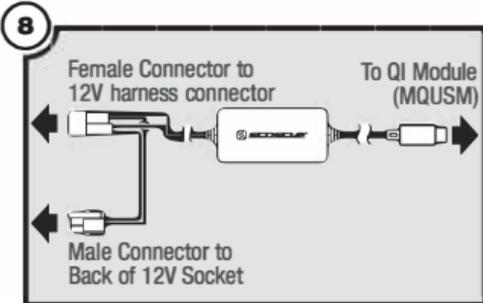
9. With the power connected to the t-harness, route the type-c connector under the shifter panel and through the hole created in the preparation step on page 5, and lastly through the HAQ02 Qi bezel. Note: Tuck away any excess cable under shifter panel, away from the shifter.
