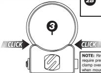
NOTE: Ring clamps 2" & over in size may require pre-stretching to help spread the clamp over the tube. (Use Protective film when mounting)
