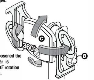
**NOTE:** When loosened the angle of the bar is capable of 360° rotation for positioning.
