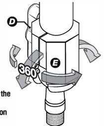
**NOTE:** When loosened the angle of the bar is capable of 360° rotation for positioning.
