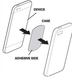
**NOTE:** If you choose not to attach the metal plate to the device or case please leave the adhesive backing in place. Position the plate between the device and interior of case with the metal surface facing the case.
