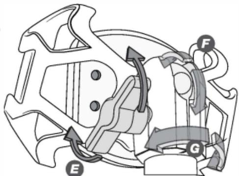
**NOTE:** When loosened the angle of the **MAGICMOUNT™** is capable of 360° rotation for positioning.
