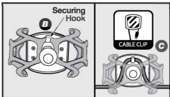
Note: Securing hook can also be used as a cable clip when elastic band is not being used (**C**).
